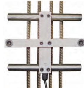
The LMC intelligent wire rope sensor is a precise device for monitoring the load in traction elevators. It mounts across all hoist ropes in as little as five minutes - calibration is automatic and no test weights are required. It's perfect for both modernizations and for new installations.
