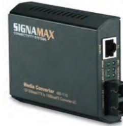
Signamax tx/rx units accept 10/100BaseT electronic signals through RJ-45 jacks and convert them for duplex (two-way) optical transmission over either 62.5µm or 50µm multimode fiber and ST and SC connectors. The system consists of two units, power supplies and patchcords. Call for other configuration options.
