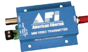
American Fibertek M100C units are compact video converters that transmit one-way from cab to security center. They can operate over either 62.5µm or 50µm multimode fiber with any camera with a coaxial output. ST and SC versions are available. The system consists of a tx/rx pair with power units and patchcords.
